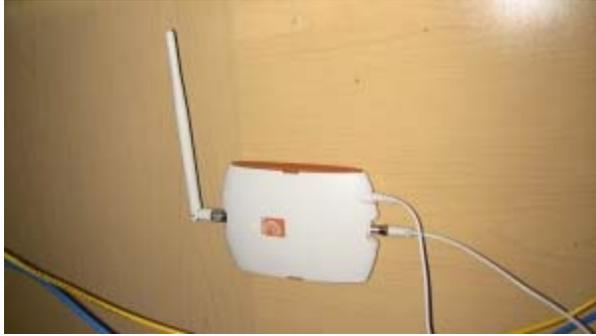
Once everything is connected, plug in the power supply, and wait up to 60 seconds for the units to start broadcasting the signal. Use the LED indicator and the chart below to ensure your unit is functioning properly.
