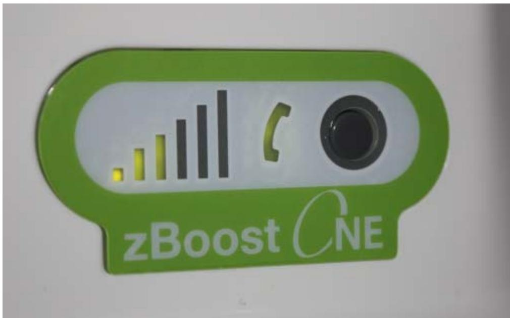
Finally, use the Signal Strength Indicator to find a location that has 3 or more lit bars to provide the optimal performance for the base unit.
