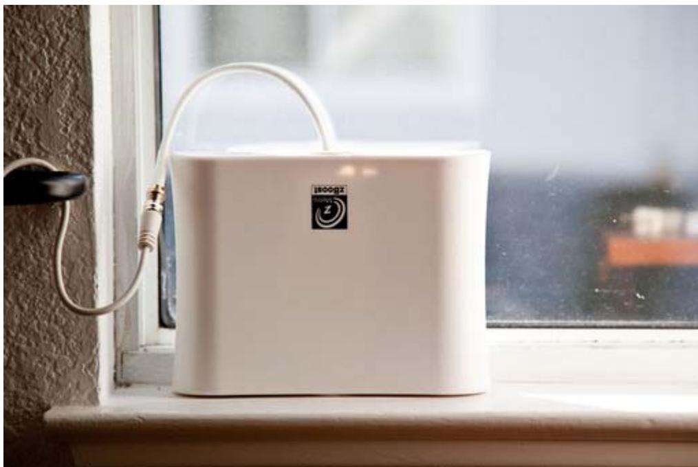
*The signal antenna for the zBoost Metro in my window sill. Since this device doesn't require vertical separation like other single amplifiers, you can even use it in a single-level apartment or small office.*
