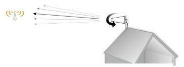
The wide band directional stretched log periodic signal antenna provides increased coverage for all cellular bands (700MHz - 2700MHz) when aimed in the direction of your carrier's signal.
