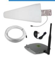
Wi-Ex, the leader in consumer cellular booster kits, now offers the YX560SL to provide increased in-building voice and data coverage for superior reach into rural environments. The YX560SL supports multiple users and all devices operating on (CEL) 800MHz and (PCS) 1900MHz.
